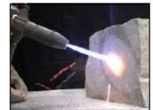
SPALLATION Drilling for Deep Heat Mining rothenfuh @ipe.mavt. ethz.ch, ETH Zurich July 2, 2007
